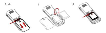
Figure 10 Battery replacement
